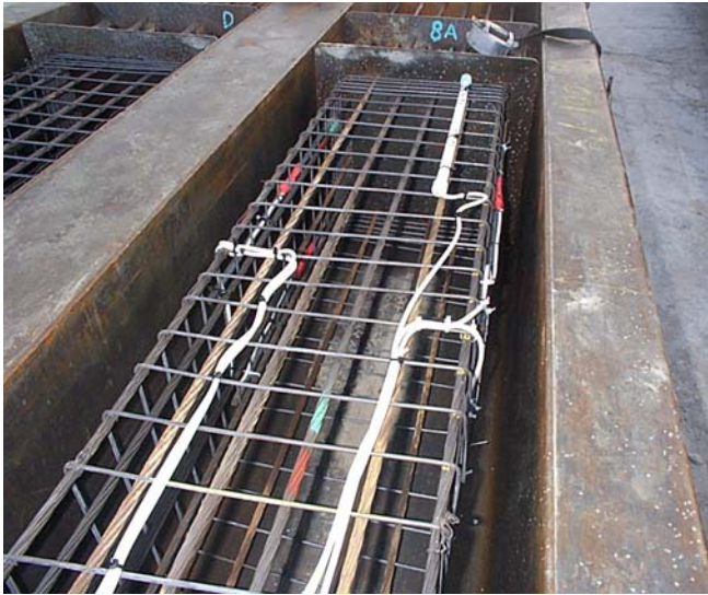
Sisterbar resistance strain gage and toe accelerometer instrumentation for prestressed concrete pile.
