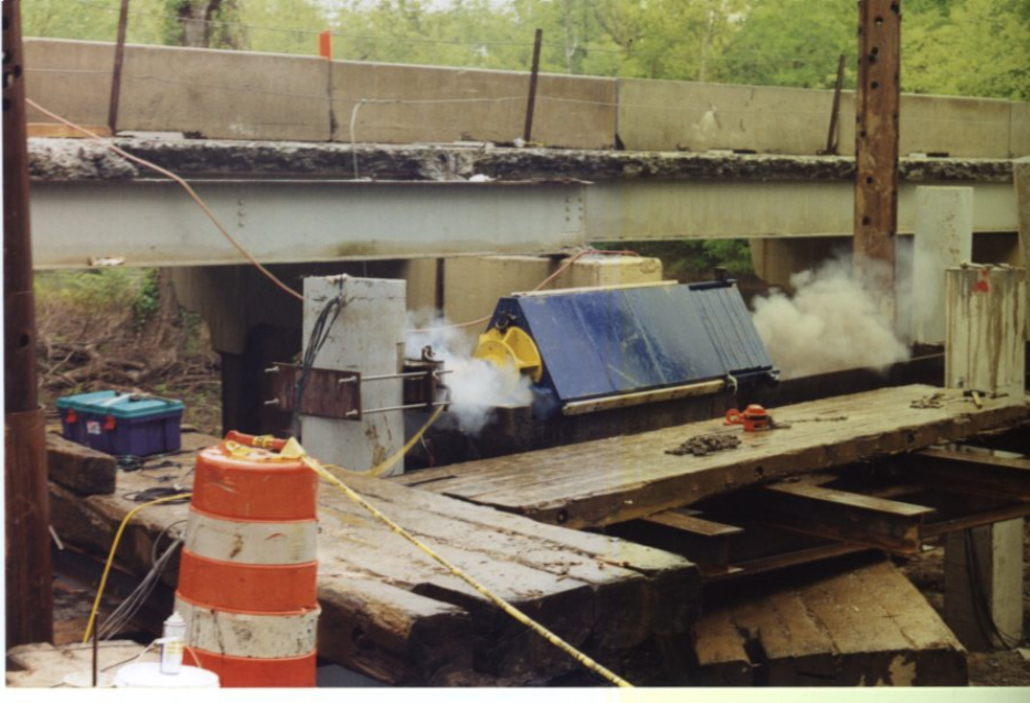
60 ton lateral Statnamic load test on a driven pile (Route 40 over Nottoway River – Virginia Department of Transportation).
