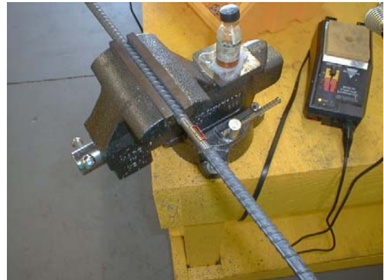
(below) Sisterbar resistance strain gage instrumentation for drilled shaft foundations.
