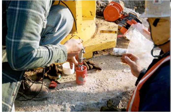
Downhole Lateral Motion Sensors (DLMS) at left being installed in inclinometer casing at right.
