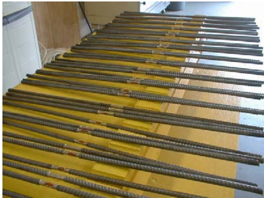
(below) Sisterbar resistance strain gage instrumentation for drilled shaft foundations.
