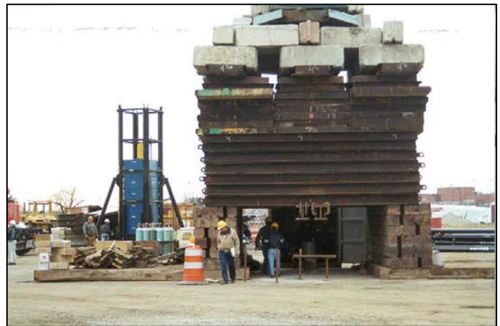
(Right). Comparison of 500 ton static test and 500 ton Statnamic load test. (Newark Airport)
