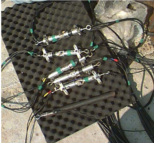
Downhole Lateral Motion Sensors (DLMS) at left being installed in inclinometer casing at right.
