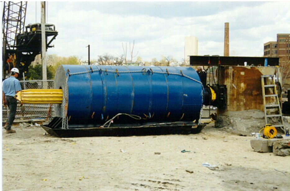
60 ton lateral Statnamic load test on a driven pile (Route 40 over Nottoway River – Virginia Department of Transportation).
