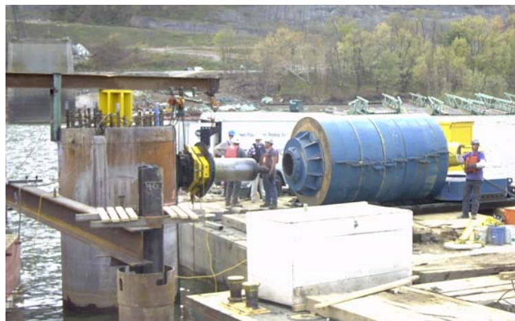
Catch mechanism STATNAMIC load testing amongst a forest of Augercast piles. Daytona Beach, Florida
