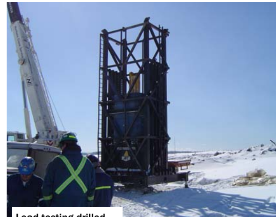
Load testing drilled shafts with 16 MN Catch mechanism Ft. McMurray, Canada (600 miles north of Montana)
