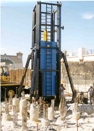
Catch mechanism STATNAMIC load testing amongst a forest of Augercast piles. Daytona Beach, Florida
